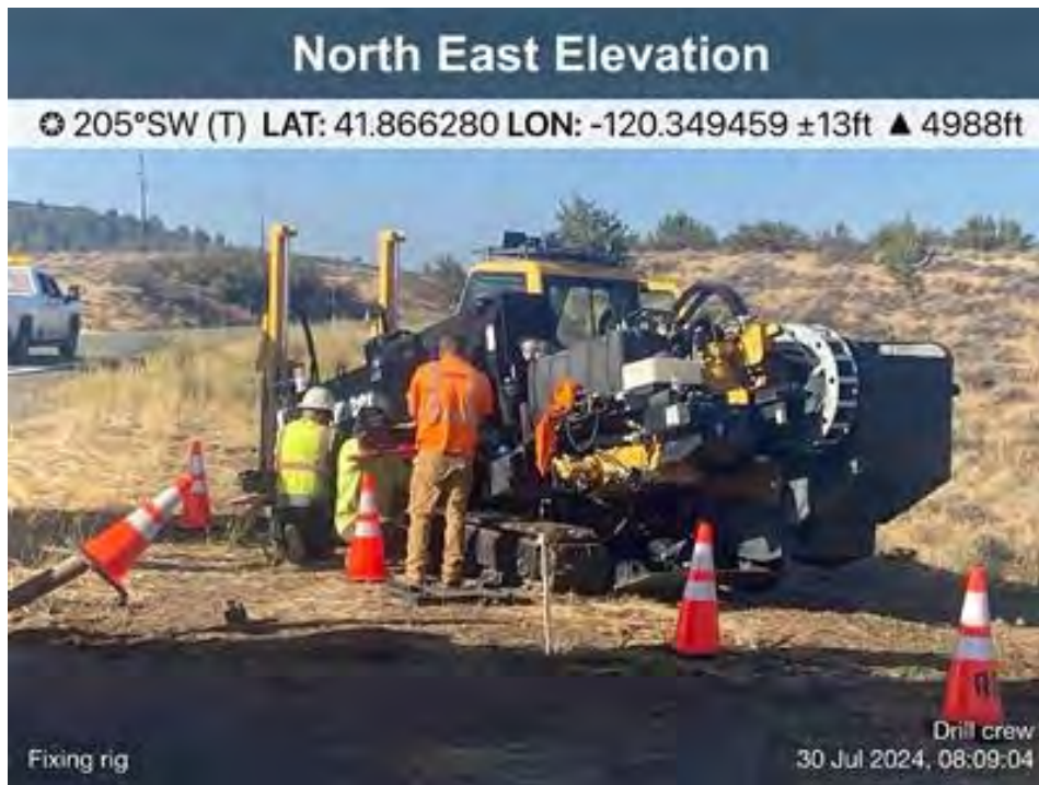
Figure 12. View to the southwest of crew doing maintenance on a drill rig in the Northern Area (Modoc County).
